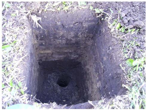
Figure 6-1: Auger Test In Banded Fill
