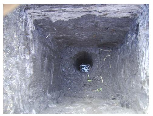
Figure 6-2: Auger Test In Banded Fill At Water Table
