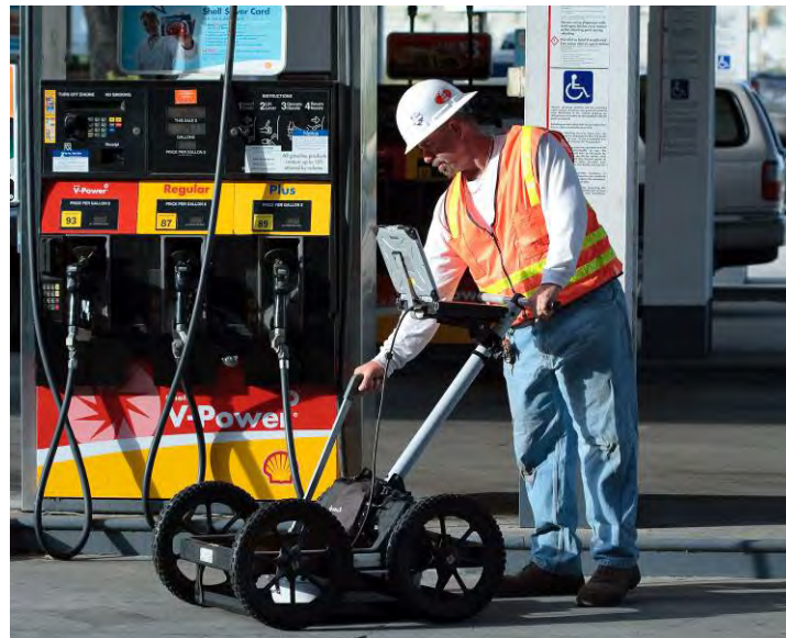
Marking fiberglass fuel lines with GPR
